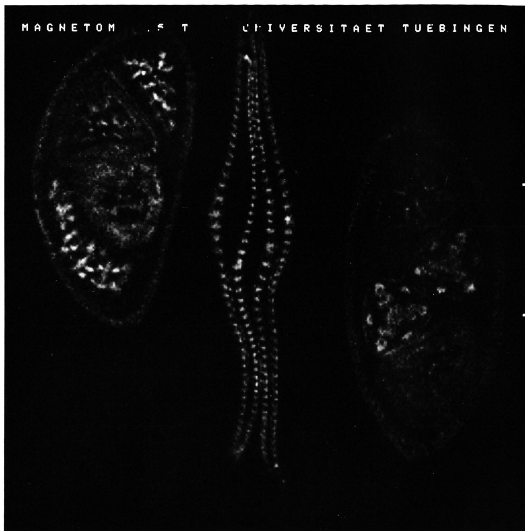
Fig. 5. High-resolution image of the inner part of an Amaryllis bulb from above with growing leaves in the middle and two blossoms, recorded by the headcoil. FOV = 40 mm, pixel resolution 156\ \mu\text{m} \times 156\ \mu\text{m} , TE = 27 ms, TR = 1 s, slice thickness 1.5 mm, 16 acquisitions, measuring time 68 min.
